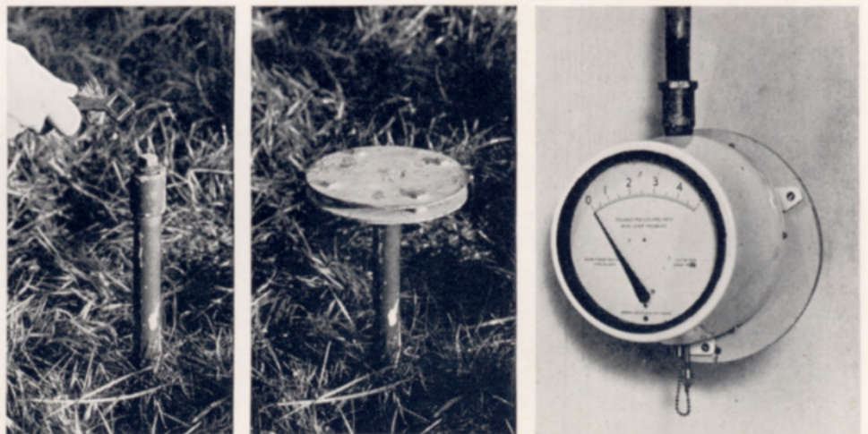
Fig. 4. Blast pipe with cap in position. This is unscrewed with the cock wrench. Fig. 5. Baffle assembly in position on blast pipe. Fig. 6. Indicator unit attached to extension pipe and screwed on the wooden disc on the wall of the post. Note the drain tube cap in position. The reset button is visible just in front of the drain tube.
