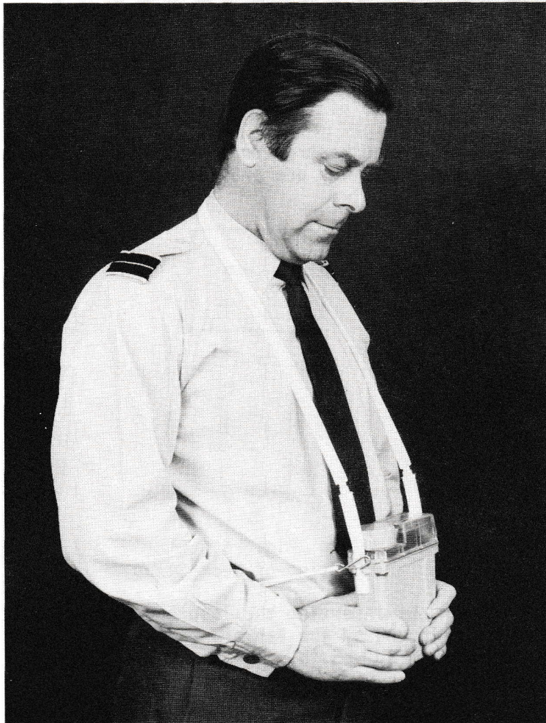
Fig. L5.5 Instrument worn with neck strap and lanyard correctly adjusted
