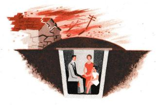
A slit trench with earth covering protects against blast and radiation
