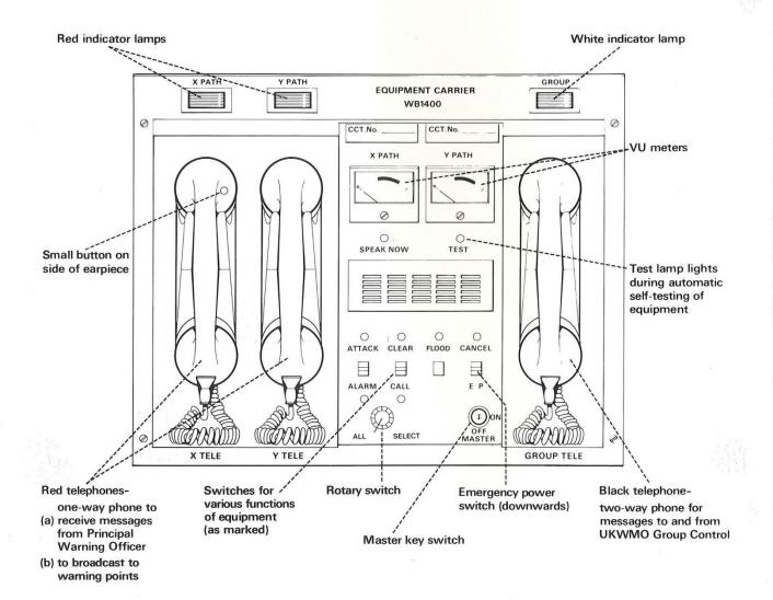
DIAGRAM OF CARRIER CONTROL EQUIPMENT
